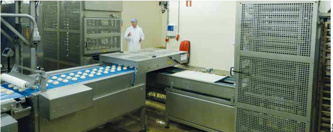
++ The filled dough pieces are deposited onto trays. Input and removal take place automatically. The entire project was designed by the Kortlever company
